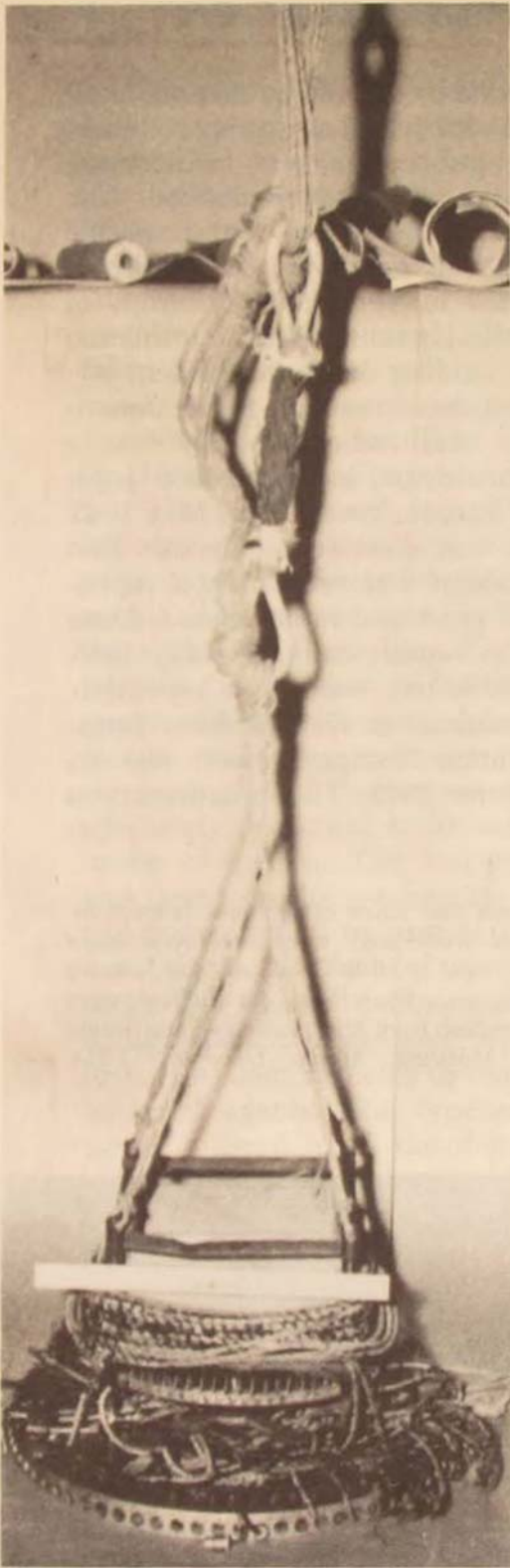
The Holy Cross balloon had this altitude device suspended from it. The section linking two knotted portions of rope shrouds is composed of numerous light rubber bands, to act as shock absorber.
